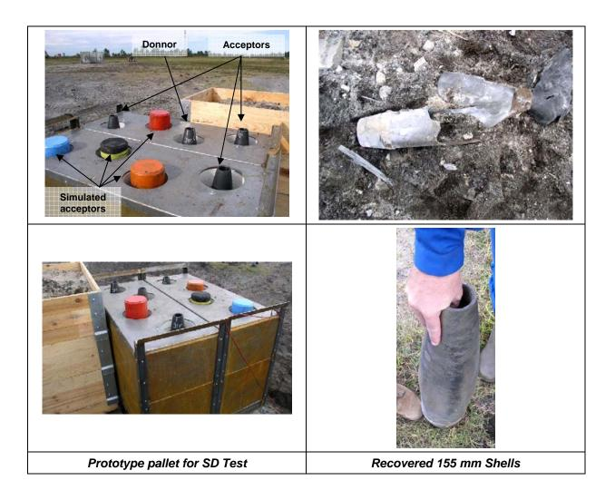
The results have shown the absence of sympathetic detonation in standard conditions between internal items and between pallets. The recovered acceptors are shown on the picture above. The nearest acceptor is partially torn, the two others are intact.
